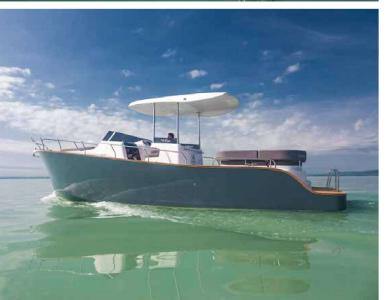
N° OF BOATSSeveral unitsAPPLICATIONPleasure boatLOA10 mDISPLACEMENT4.6 tELECTRIC MOTOR2 x 15 kWBATTERY10 kWhYEAR
