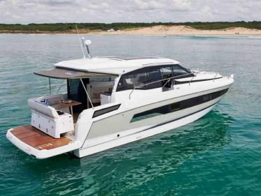
N° OF BOATS1APPLICATIONPleasure boatLOA11.47 mDISPLACEMENT6.8 tELECTRIC MOTOR2 x 35 kWBATTERY2 x 30.8 kWhYEAR2019
